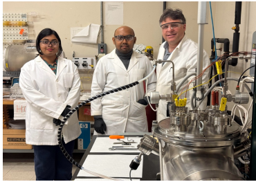
Researchers deposit cadmium telluride thin films to understand how the controlled incorporation of parts-per-million additional elements can improve their electronic properties in solar cells.
